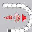
EVOSILENCE® Noise damping in side link Noise reduction of up to 10 dB(A) with damping elements in the chain links.
